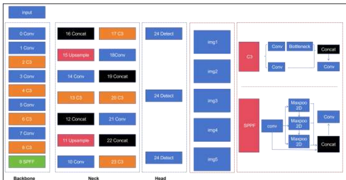
Figure 2 YOLOv11 network structure diagram
