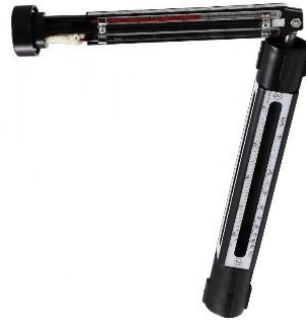
Figure 1 Basic Structure of Whirling and Sling Hygrometers
