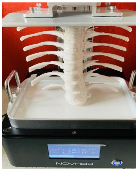
Figure 1 Photopolymerized 3D-Printed Thoracic Vertebra Model
