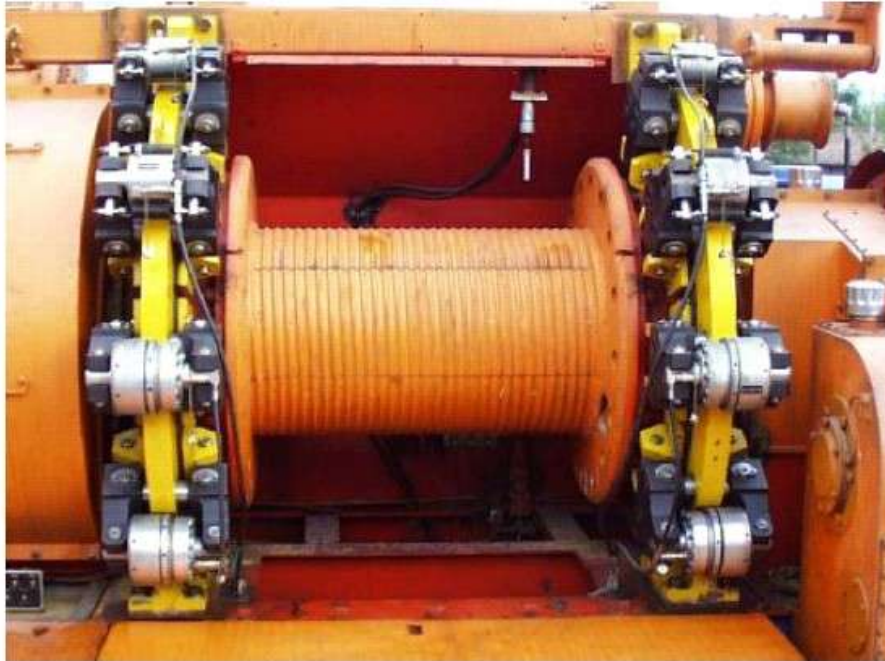
Fig.1 Oil drilling rig hoisting winch and brake mechanism
