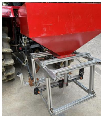
Figure 6 - Fertiliser drainage validation test
