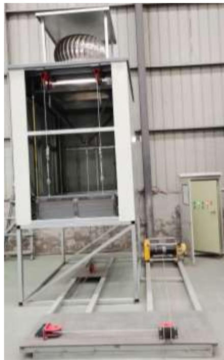
Fig. 2. Principle prototype of the passive ventilation device
