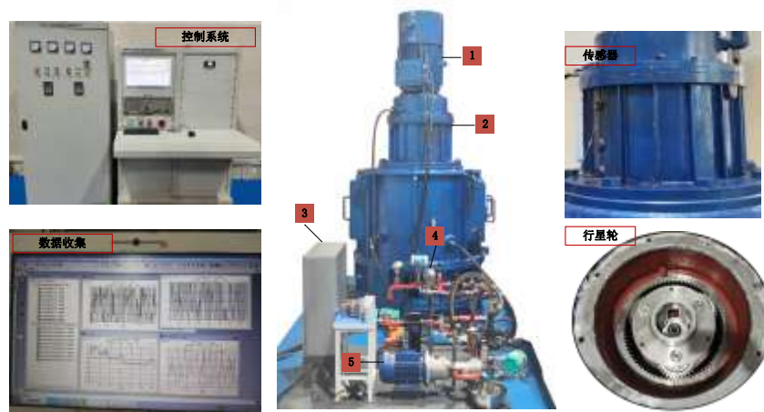
1 - Input motor, 2 - Planetary gearbox, 3 - Distribution pump, 4 - Oil pump of lubrication system, 5 - Motor of lubrication system
