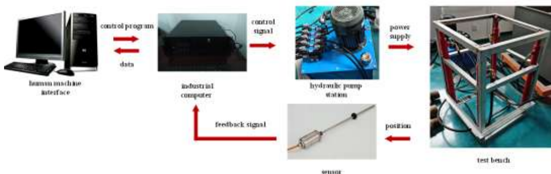
Figure11 Hydraulic system control experiment schematic diagram for frame lifting
