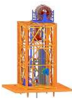
(a) Schematic of the frame in lowered position
