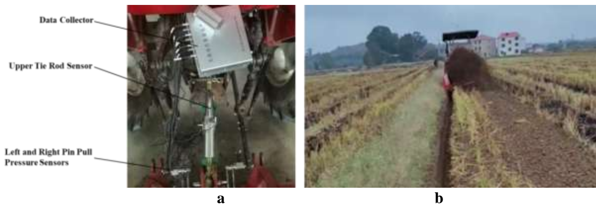
Figure 7. Field validation test. (a) Installation position of the telemetry system; (b) Ditching test
