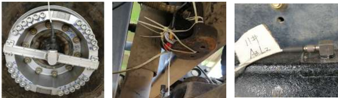
A. Six-component force sensor B. Pull wire displacement sensor C. Acceleration sensor
