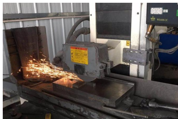
Figure 2 Grinding hardening process
