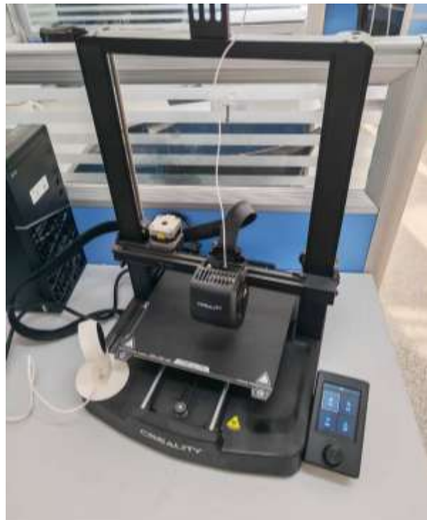
Fig. 1 FDM additive manufacturing and visual system experimental platform.
