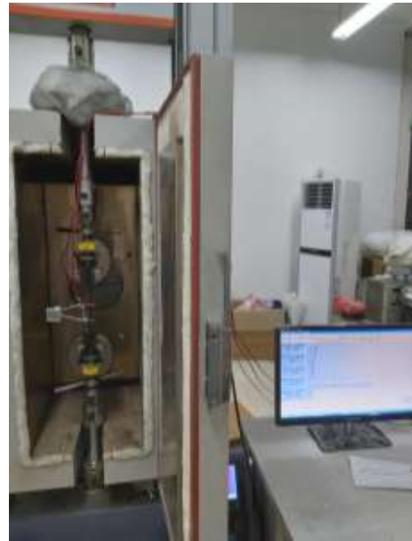
Fig 5 Experimental set-up for CTD testing
