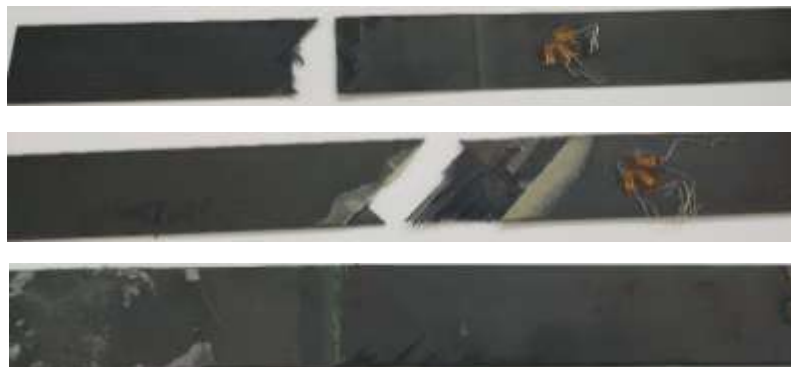
Fig 6 Failure modes in repaired specimens
