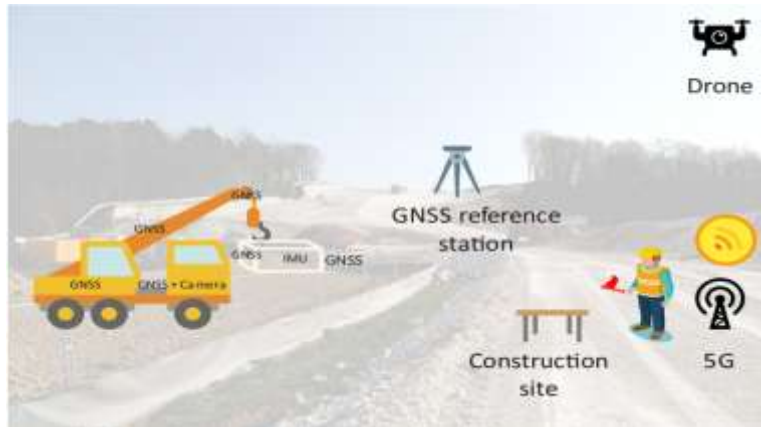
Figure 1: System overall architecture
