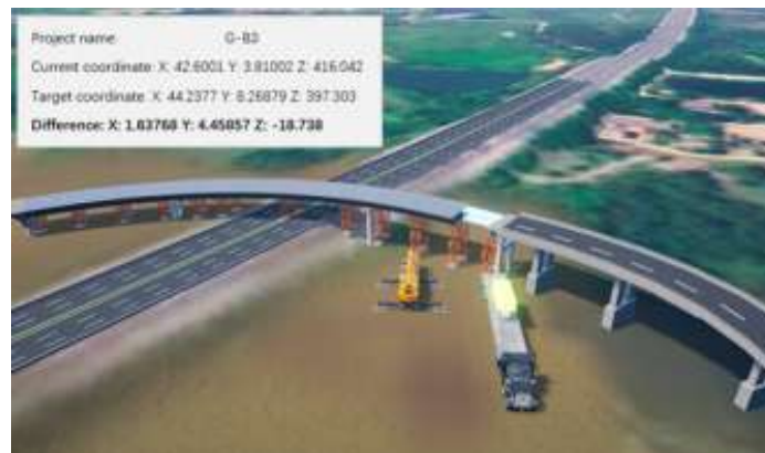
Figure 4: System front-end with sensor data
